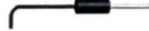
VP5 blunt needle, 90 degree and delivery laser Doppler probe for assessment of rear teeth
